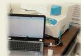
Rapid Visco Analyzer (for analysis of starch pasting properties.)
